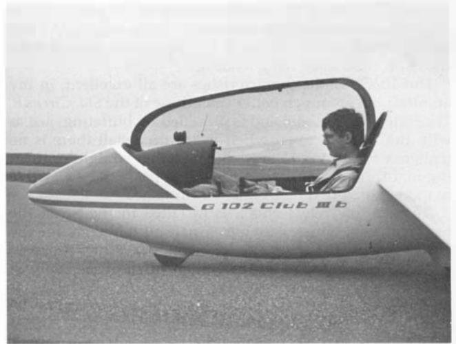
At six feet two inches, test pilot Bruce Beddow fits nicely into the Club IIIb, whose faired nose wheel allows for heavy braking on landing.
