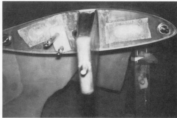
Left wing root showing areas where major air leakage was corrected.
